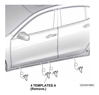
22. Remove the adhesive backings while lightly pressing the rails against the vehicle. Using the palm of your hand, firmly press the rails against the vehicle panel for 30 seconds. Remove the marks you made using isopropyl alcohol on a shop towel.
